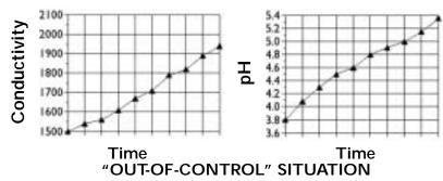
These two graphs represent a drastic contamination situation. The conductivity, and probably pH, keeps on rising rapidly. Thus, the level of contamination is increasing faster than fresh solution is being added.
