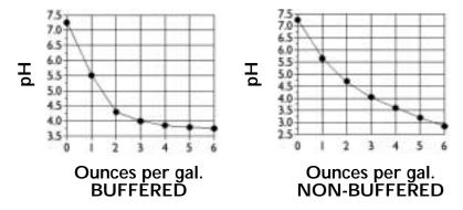
Notice that the buffered curve flattens out near pH 4.0 and then changes only slowly. On the right, notice that the pH is not very stable as more concentrate is added—the pH just keeps going down.
