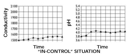
Notice that the pH and conductivity rise slightly after a few hours and then level off to a fairly constant value. This is very normal and represents minor contamination.
