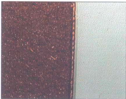
Strippable blankets surface: the top printing face and non-printing black area are evident. Photo Reeves.
