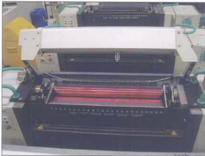
Ink hood open to show ink fountain agitator that prevents high-tack UV ink from standing still in the ducts. Photo: MAN Roland.
