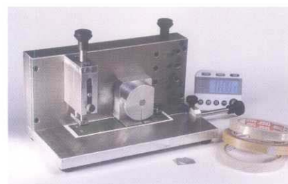
FOGRA's LHT adhesive tape scratch resistance test measures values automatically.
