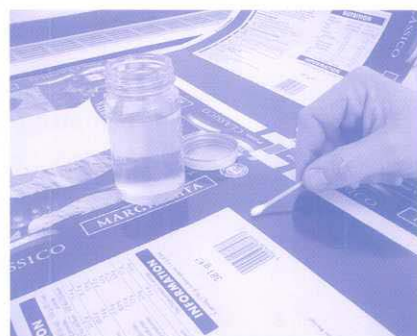
The traditional method to test if printed sheets have been adequately cured compares resistance to solvent attack between a printed sample and a standard test sample. Source Sun Chemical.
