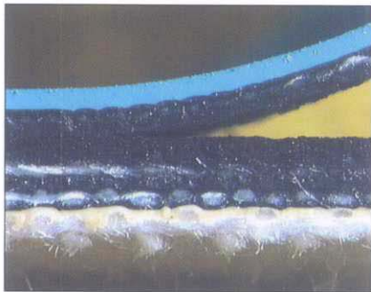
Use blankets with open cell compressible layers to make stripping easier. Photo Reeves.
