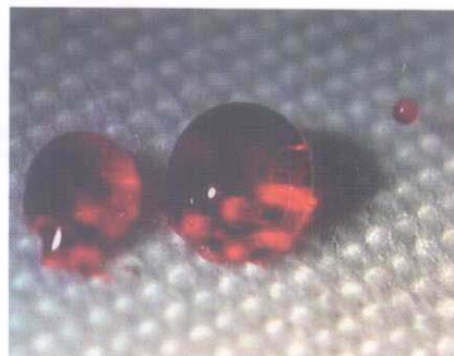
Water solvent protection of blanket fabrics protects them against penetration by solvents, additives and other chemicals. Photos Reeves.
