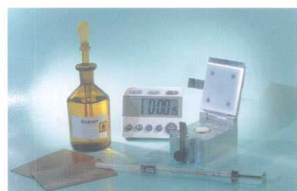
ACET is a simple to use solvent resistance test device developed by FOGRA
